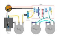
The instrument reconfigures existing circuits; a fixed system comprising of three modules:Noise Siren, Quad Sine, and Flub Filter. The design process involved modifying existing equipment: circuit bending [2][3] (na "ive play) and hardware hacking [4] (informed intervention).
